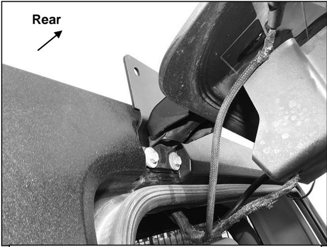
**(Fig 6) Slide Rear Window Bracket between the hinge and the top. Do not remove factory bolts**
