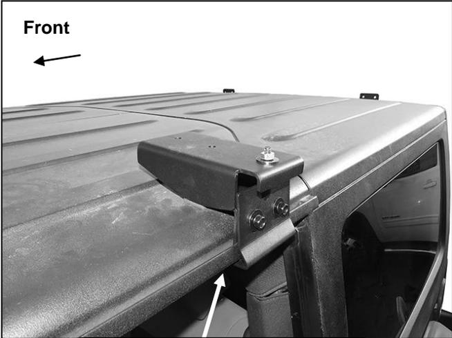
**(Fig 4) Slide the Clamp Bracket under the rain gutter (arrow)**
