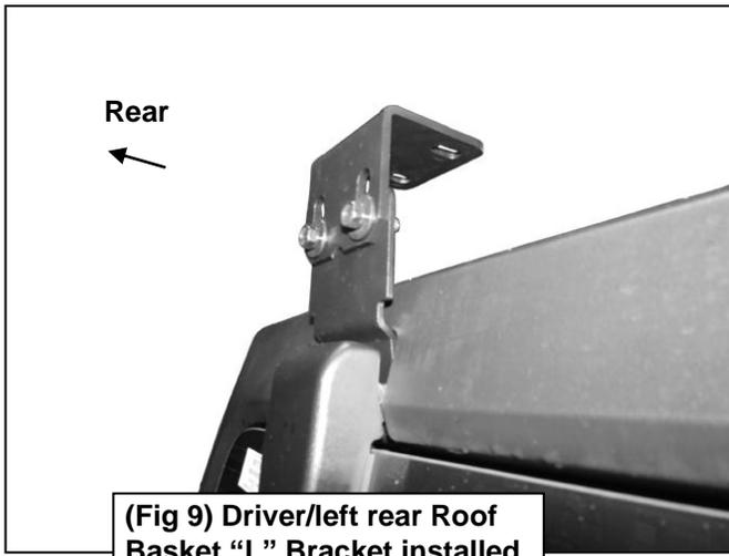
(Fig 9) Driver/left rear Roof Basket "L" Bracket installed
