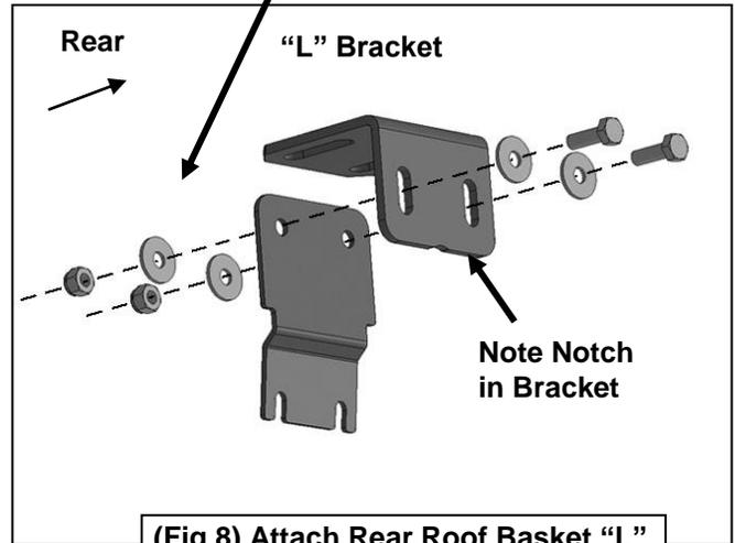
(Fig 8) Attach Rear Roof Basket "L" Bracket to Rear Window Bracket
