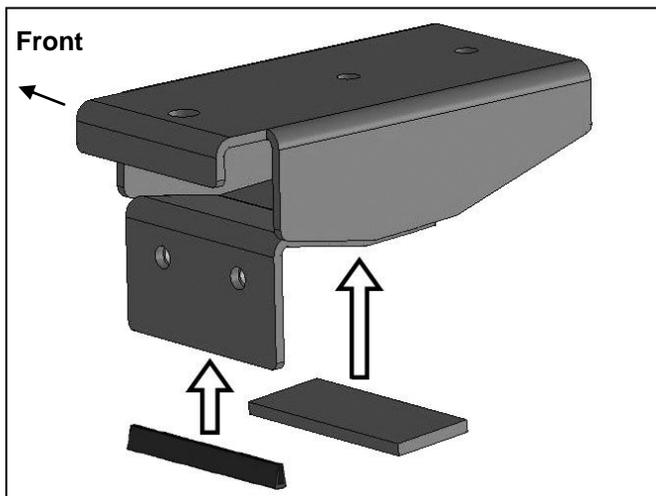
**(Fig 1) Attach Foam Pad and Edge Trim to bottom of Bracket**
