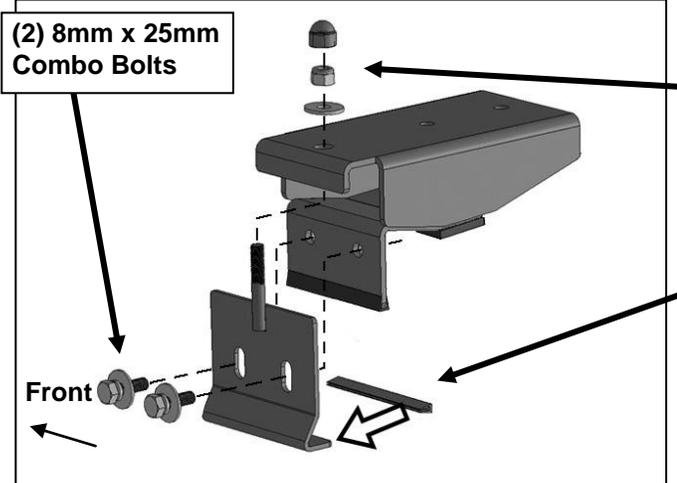
**(Fig 3) Attach Clamp Bracket to Mounting Bracket**
