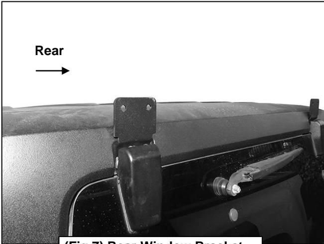
(Fig 7) Rear Window Bracket installed on driver/left side
