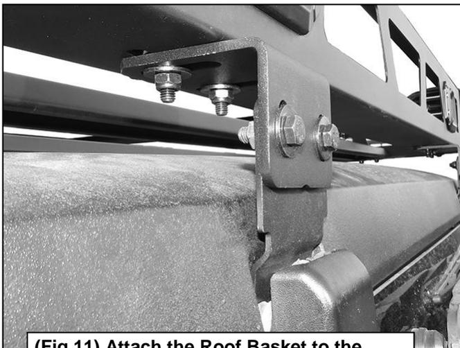
(Fig 11) Attach the Roof Basket to the Rear "L" Brackets (driver side pictured)
