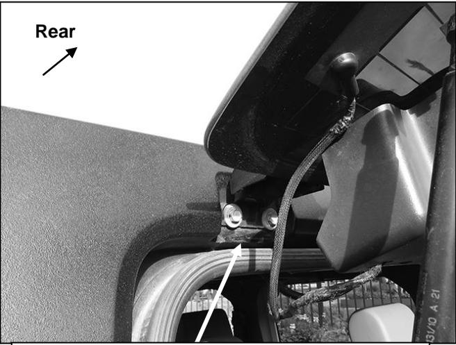
**(Fig 5) Open rear window. Loosen but do not remove (2) rear window hinge bolts (arrow)**
