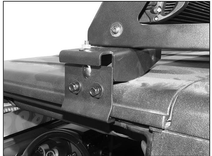
(Fig 10) Slide Bracket assembly forward or back to line up with Basket. Attach Basket to the Front Brackets (driver side pictured)
