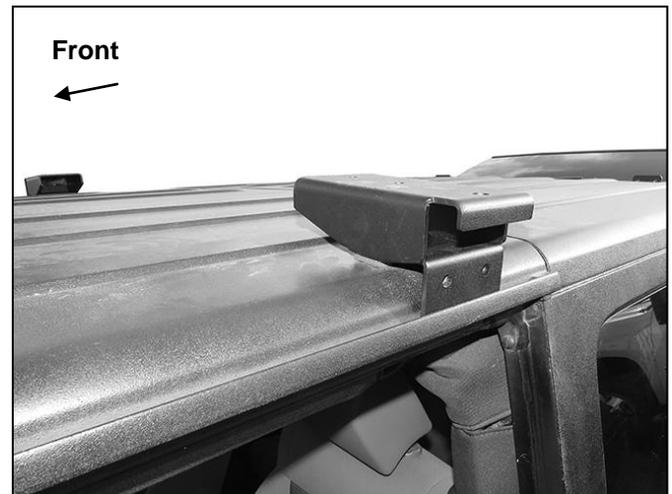
**(Fig 2) Place the tab on the Bracket inside the rain gutter (driver side 2dr model pictured for instruction purposes only).**
