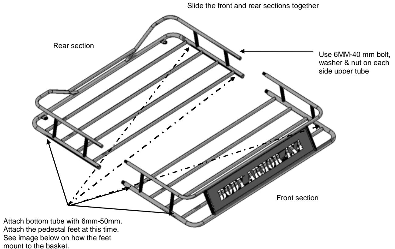
1. Join the front and rear sections of the basket. Use 6MM-40MM bolts on the upper joint.
