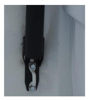
4 Locate and install middle support legs in top holes of cab basket and at bed side channel locations.
