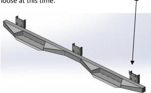
4 Check alignment to body and tighten hardware.
