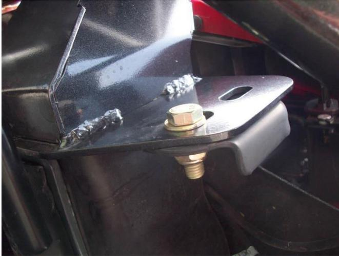
Insert flat plate from the bottom, Line the nut with the center hole
