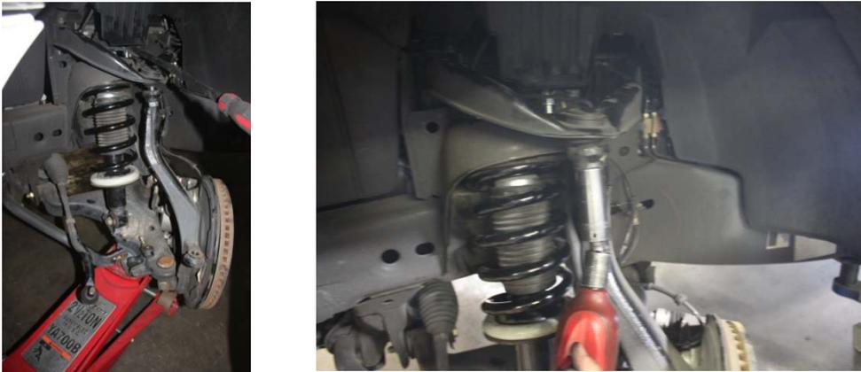
8. Repeat steps 1 through 6 on the passenger side of the vehicle, then re-install the sway bar nuts on both sides and re-torque to the factory specs.
