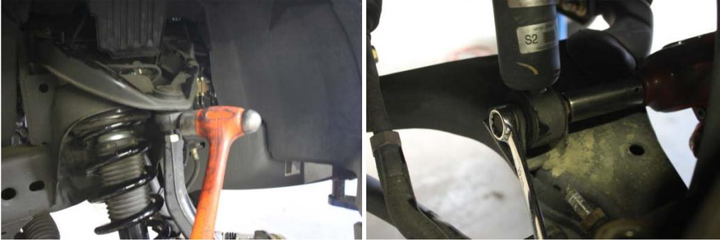
4. Remove the strut from the vehicle and mount it in a bench vise, and install the strut spacer. Torque fasteners to OEM specification. Note the shape of the spacer, the strut will be rotated 180 degrees when installed.
