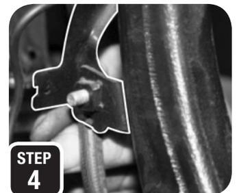
**STEP 4 :** Next, remove the clip at the upper ball joint nut, loosen the nut but do not remove, and break the ball joint loose by hitting the side of the spindle with a hammer. The nut will catch the spindle, then remove the nut (*never hit the ball joint on the threads*).
